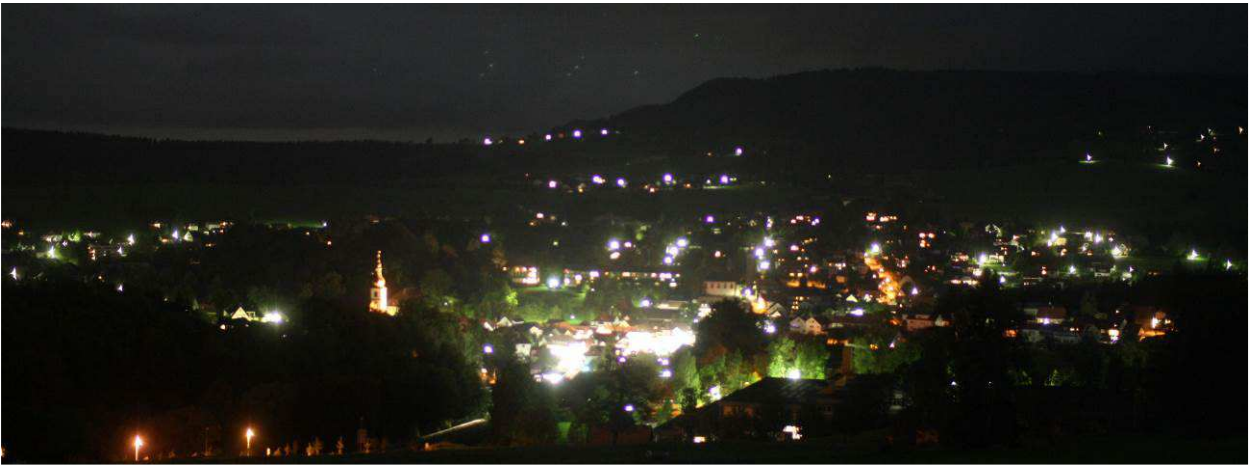
Fig. 7.8: Gersfeld: Mainly badly shielded lights in the center (ULR=11.6%, 1746 klm)
