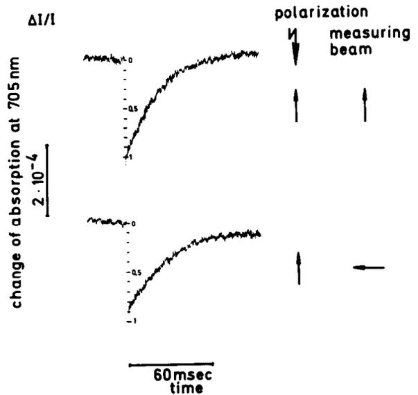
Fig. 2. Flash induced absorption changes of chlorophyll- $a_1$  at 705 nm: Above, exciting and measuring beam polarized in parallel to each other; below, exciting and measuring beam perpendicular to each other; standard reaction medium;  $T = 20^\circ\text{C}$ ; viscosity, 1 cPoise, average over 320 signals; repetition rate 4 Hz; intensity of the measuring beam: 600  $\text{erg}/\text{cm}^2/\text{sec}$ , excitation at wavelength greater than 690 nm, 20% of saturation.
