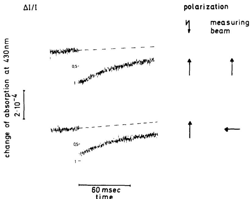
Fig. 3. Flash induced absorption changes of chlorophyll- $a_1$  at 430 nm. Polarization as in fig. 2: Standard reaction medium + 13% Ficoll (Pharmacia),  $T = 2^\circ\text{C}$ ; viscosity, 15 cPoise; average over 3200 signals (4 changes of the cuvette); repetition rate 4 Hz; intensity of the measuring beam:  $1000 \text{ erg/cm}^2/\text{sec}$ , excitation at wavelength greater than 690 nm, 12% saturation.
