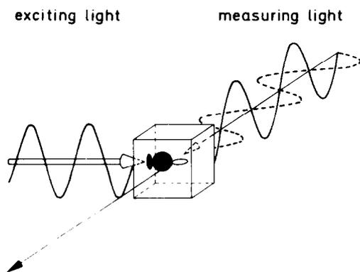
Fig. 1. The geometry in photoselection experiments. The orientation of the E-vector of the exciting and the measuring beam is indicated by sinoidal lines: Full circle, membrane orientations which lead to the excitation of in plane oriented oscillators; open circle; membrane orientation which does not lead to excitation.
